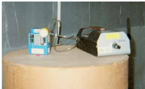
Photograph 3. 1: Air Sampling Pumps and Jerome Mercury Vapor Analyzer
